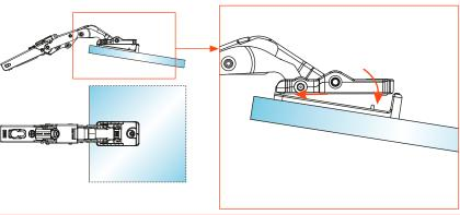
2) Locate the hinge onto the plate when it is bonded to the door.
