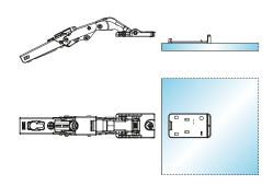
1) The hinge plate must be attached to the glass door with a specific adhesive using the correct procedure. We recommend that this operation is carried out by a specialist company. For further information on adhesives and their application, please contact the adhesive manufacturer or your glass supplier.
