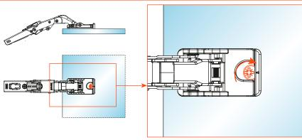
3) Rotate the fixing cam.
